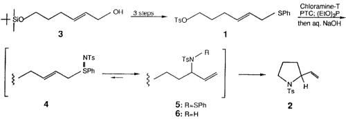
In situ amination of the phenylthio- moiety in 1 by chloramine-T institutes an allylic sulfilimine 4/sulfenamide 5 equilibrium (Scheme II). Although the equilibrium  $4 \neq 5$  lies on the side of the sulfenamide 5,<sup>7</sup> S-N solvolysis is slow under these reaction conditions and triethylphosphite is required to accelerate 5-6 conversion. Addition of aqueous NaOH (in the presence of the phase transfer catalyst) instigates intramolecular cyclization to 2.
